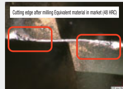
Excessive damage to cutting edge ends life of tool
