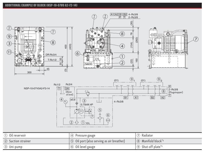
$<sup>{}^{^{1}}\</sup>mathrm{Optional}.$  When mounted on the block, shut-off plate is included as a standard.
